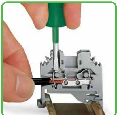
Side-entry wiring: CAGE CLAMP® connection
